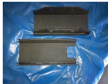
Pedestal Liner without Gap Pedestal Liner with Gap - 8329002
